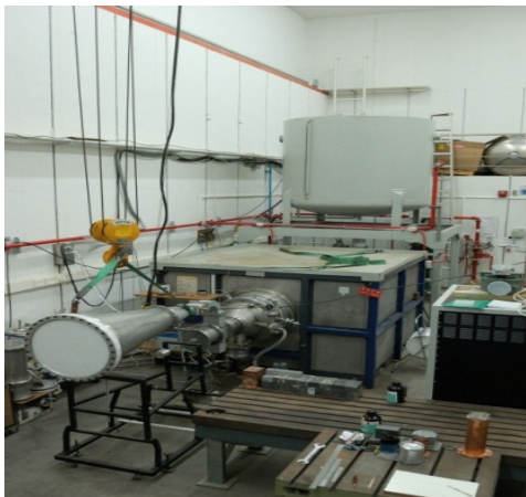
5-kJ pulsed generator 500 kV, 25 kA, 400ns
