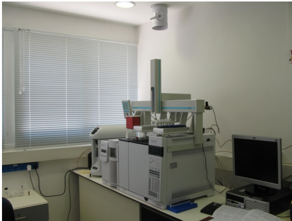
GC/MS with a Purge & Trap System For volatile organic compounds
