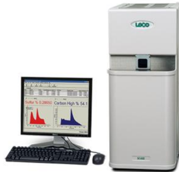
Leco unit for TC, TOC and TS measurements
