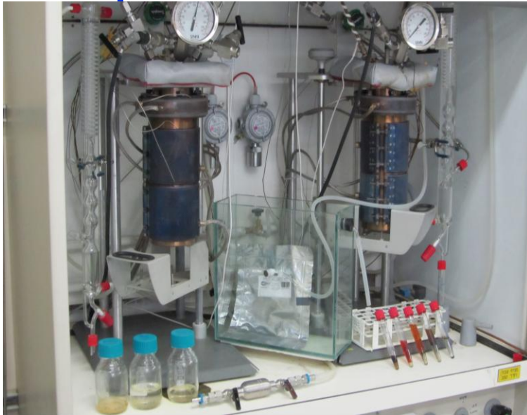
Pyrolysis reactors with oil, gas and water products
