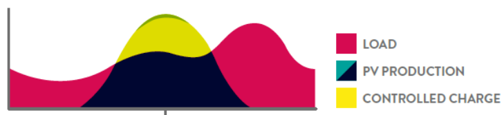
Charge control: Electric vehicle only charges when a surplus of solar power is available.
