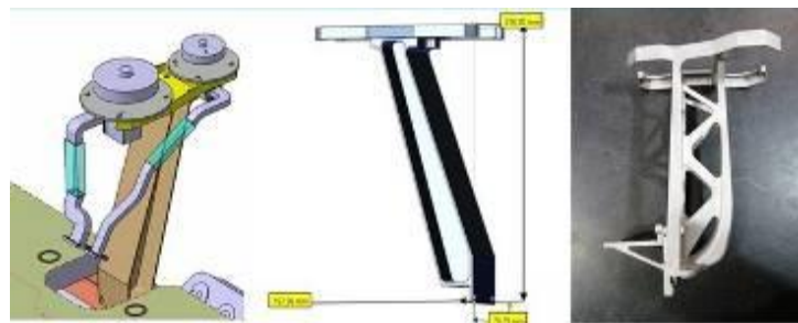
3D-printed bracket for antenna support (ESA)
