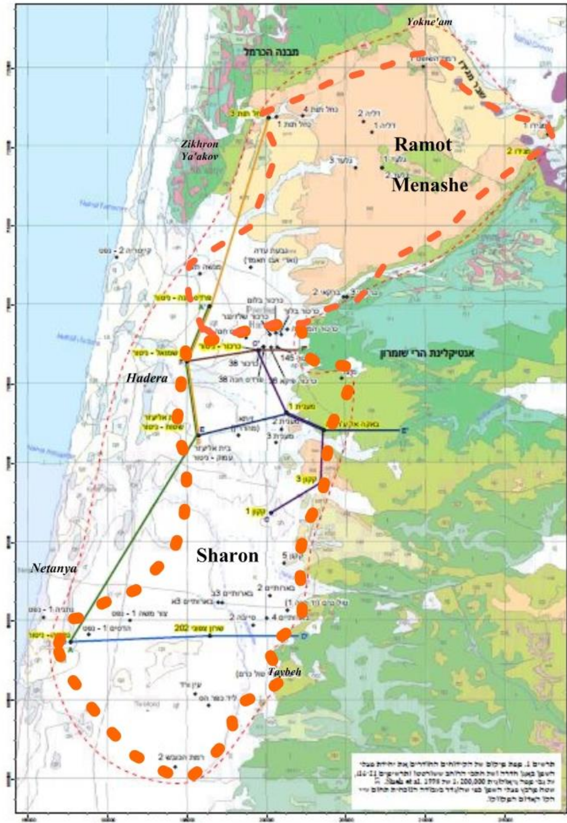
Figure 38. The oil shale occurrence in Hadera-East, as presented by Goren (2012). Proposed boundaries of this oil shale body (Sharon & Ramot Menashe occurrences) are shown in brown color.
