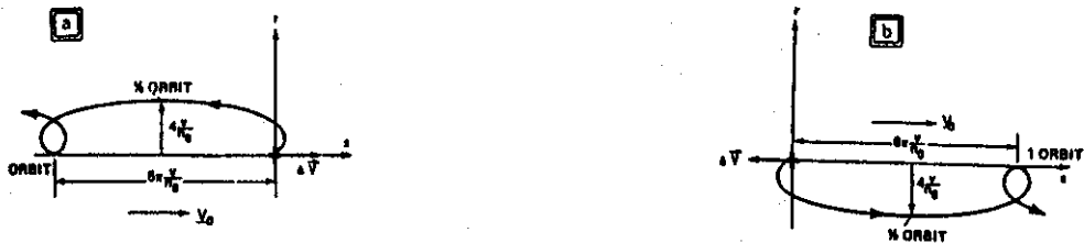
Fig. 2: Relative motion after V-bar burn a. positive V-bar burn b. negative V-bar burn
