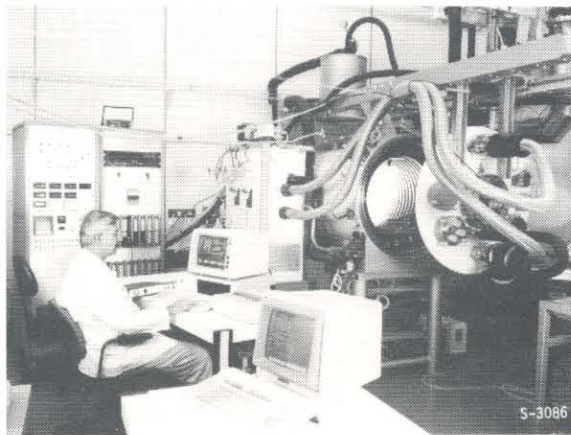
Figure 3. Activity at MBT's Thermal-Vacuum Chamber
